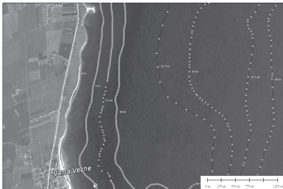
Fig. 5. Izobaths after the new data, representation with a factor of 2.5 m between lines
